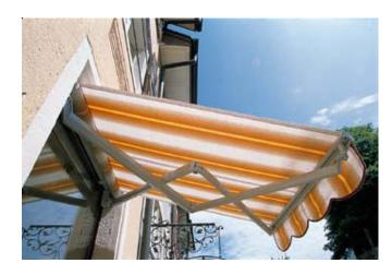
The **Trion Cross Folding Arm Awning** can be adjusted to operate from horizontal to 45°. Maximum projection is 3500mm on an awning that can be as little as 2250mm wide
